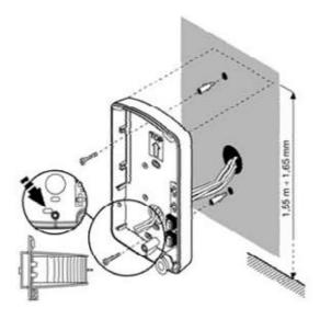
The installation is made by screwing to the wall by means of dowels.
