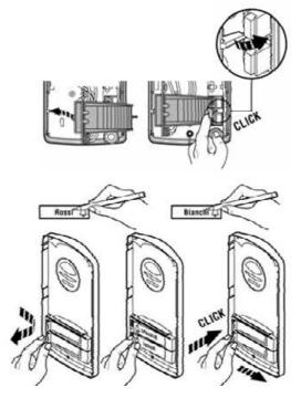
Each button has its separate nameplate hold by means of plastic flag (see figure).
